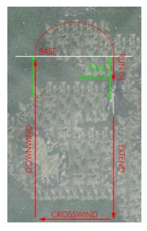
The base point is where you start your base turn and is the most crucial point in the box pattern! In the sim it is really not easy to get correct visual cues when reaching that point. A common mistake is to extend too far North before turning base. That should be avoided as it spoils the event geometry and all preset settings (dive angle, distance, aiming, ...), without mentioning the mess in the aircraft separation. If it happens nevertheless, fly a dry pass and remain at base altitude.
